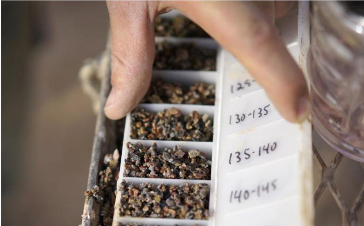
*Jeremy Vore, project geologist for Newmont Mining, looks over rock chip samples from exploration drilling at the future Long Canyon gold mine site near Elko, Nevada May 22, 2014. The numbers on the box represent the depth the sample was taken from in feet. Long Canyon is still in the exploration phase but is expected to be a multi-million ounce open pit mine by 2017. Picture taken May 22. Reuters/Rick Wilking*
