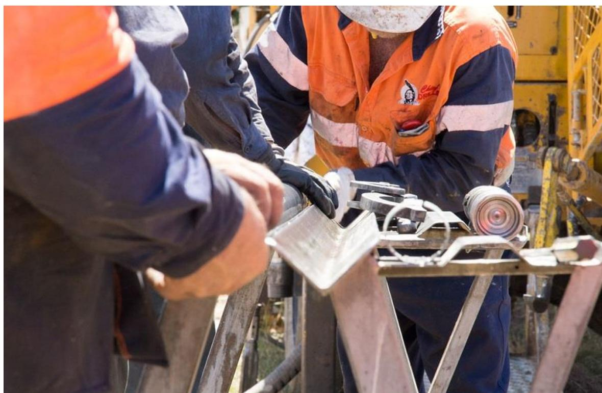
*Drill core is extracted from drill rods*
